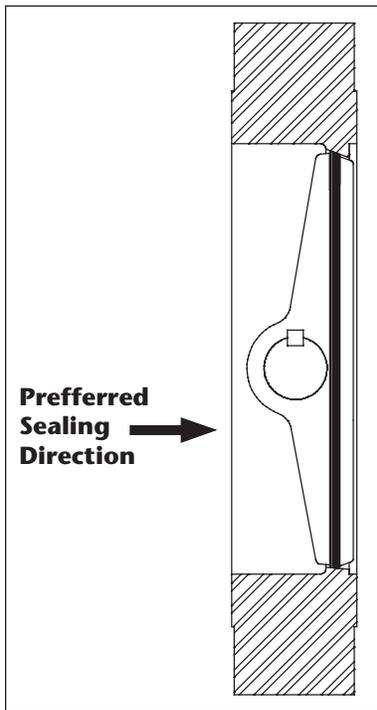
**DO NOT USE A PARTIALLY INSTALLED VALVE AS A BASE POINT TO ALIGN THE CONNECTING PIPELINE.** When one side of the valve is secured to the pipeline, the opposite valve flange may not be used to draw the connecting pipe into alignment, with the exceptions as described later in this section. Any pipe supports that maintain the connecting pipe in place must be evaluated as to the restrictive nature of the support, in regards to correct flange alignment.
