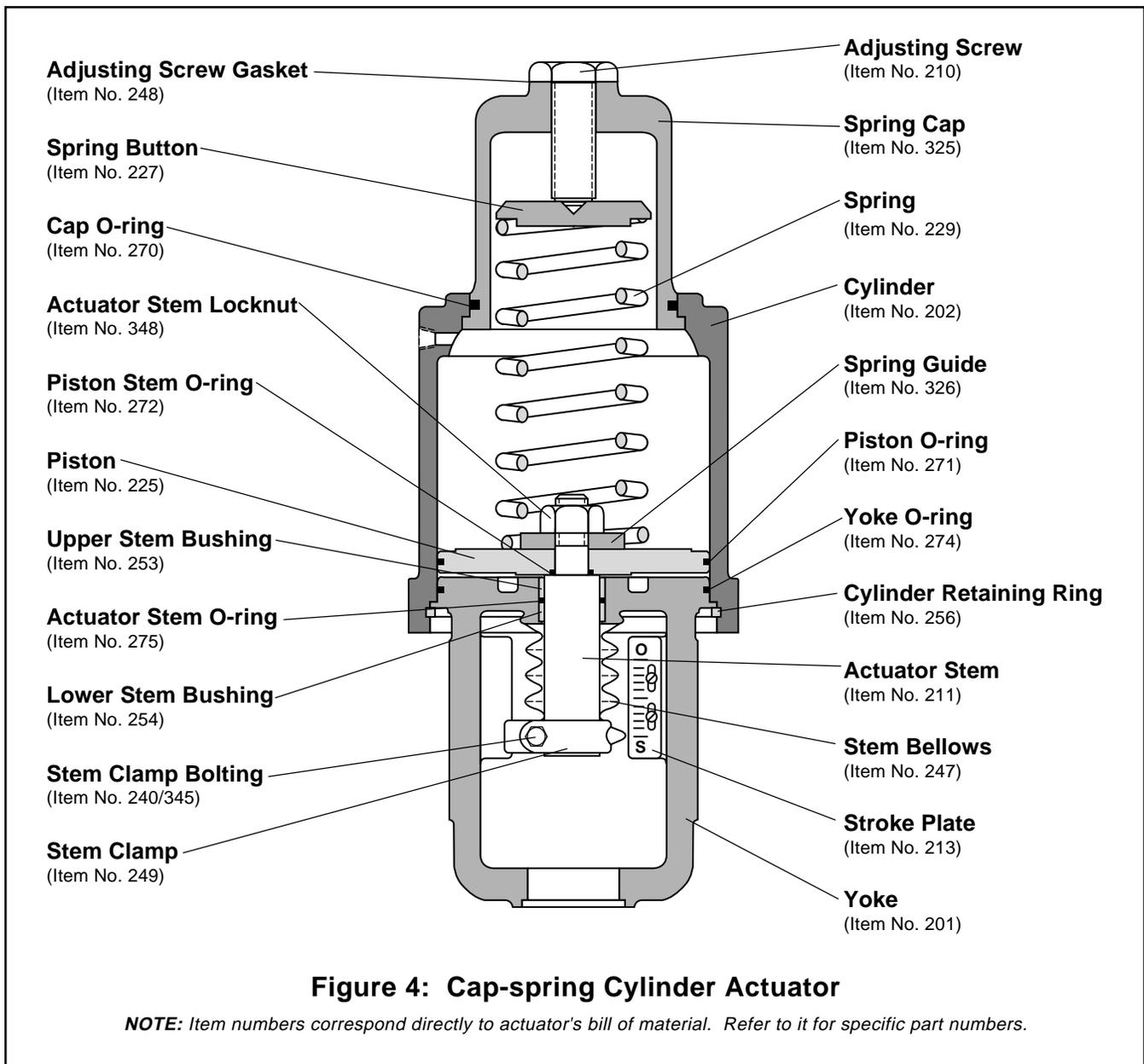
11. Tighten the adjusting screw enough to provide an air seal with the gasket. Do not overtighten.
