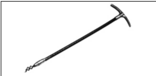
Figure 5.1A Flexible packing removal tool cork screw tip
