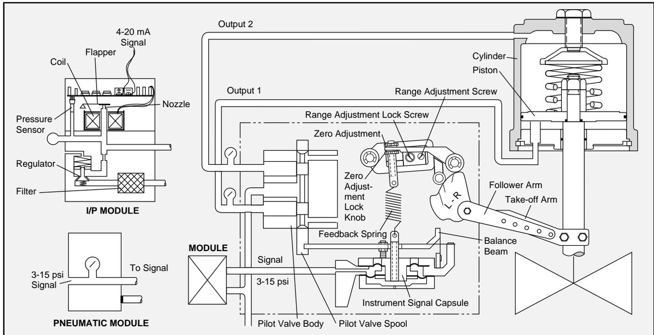
**Figure 4: Positioner Schematic for Air-to-Open (Retract)**
