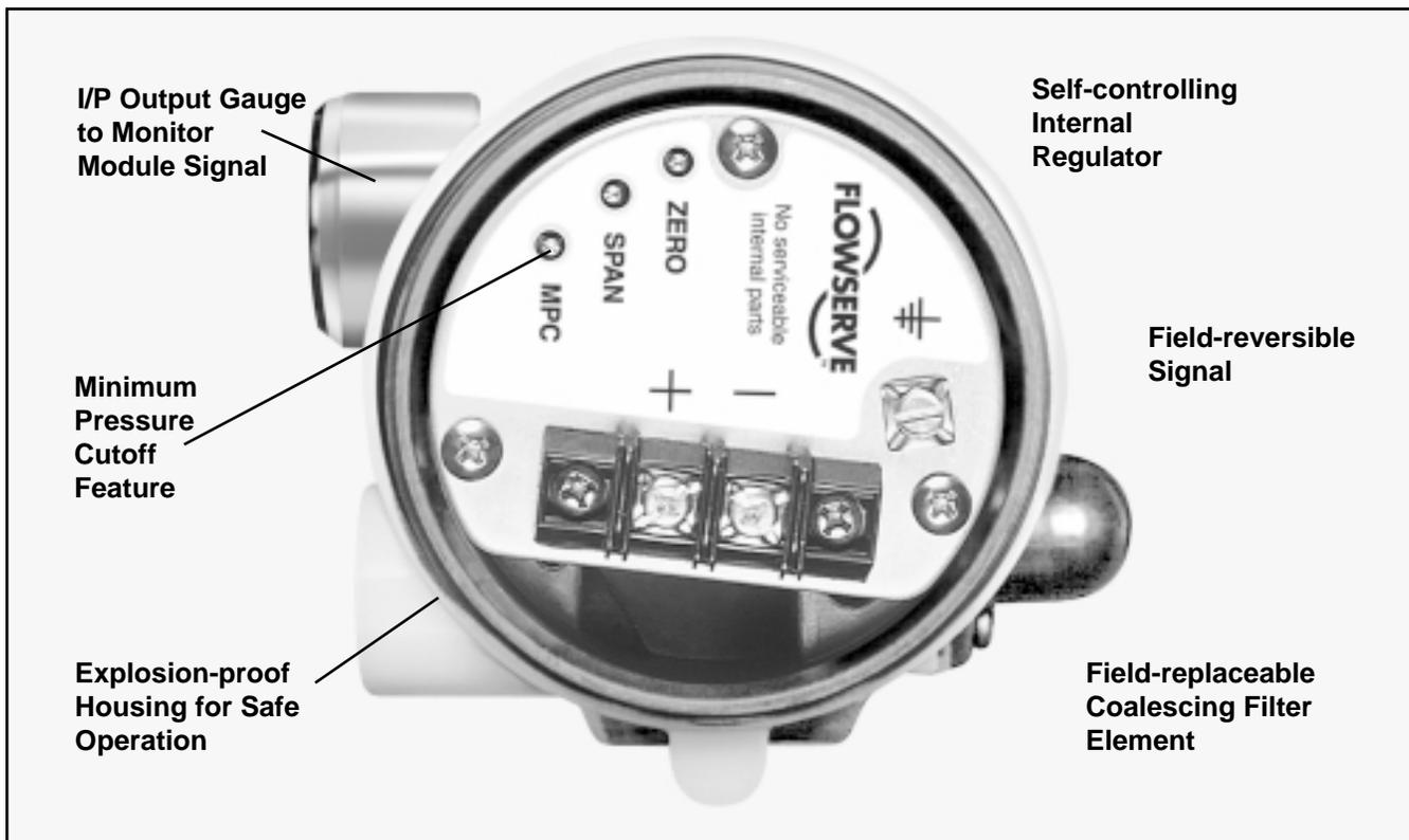
**Figure 3: Features of NT 3000 Electro-pneumatic Transducer Module**
